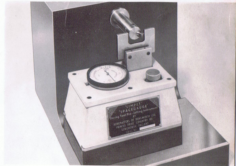
"Limpet" shown on Fine Borer set up and using the gap gauge applicable for the quantity component production purpose
